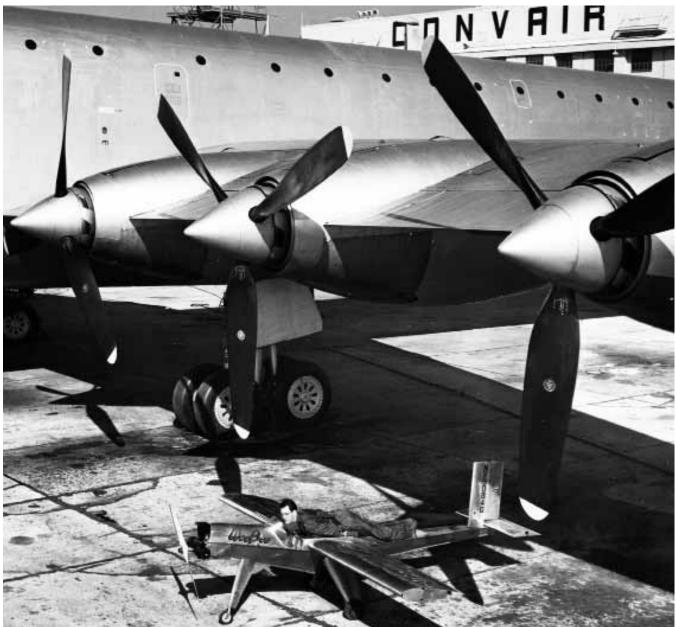
After World War II, experimenters competed to produce ever smaller aircraft. The first to be called World's Smallest Flyable Airplane was Wee Bee, shown here circa 1948 (with a pilot) on the ramp near the Consolidated Vultee facility at Lindbergh Field, San Diego. This Bee Aviation airplane had a length of 14 feet, span of 18 feet, and a 30-horse power piston engine. The pilot flew the Wee Bee while lying flat
